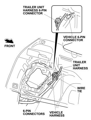
17. Secure the 6-pin connectors and trailer unit harness to the vehicle harness with a wire tie.
