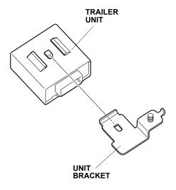
13. Secure the trailer unit to the vehicle panel with a flange nut as shown.
