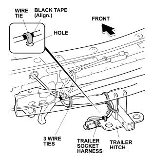
35. Secure the trailer socket harness to the trailer hitch with three wire ties.
